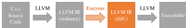
Fig. 11. Our system utilizes the Enzyme [Moses and Churavy 2020] automatic differentiation framework that operates at the LLVM level by generating differentiable versions of LLVM Intermediate Representations (IR).
