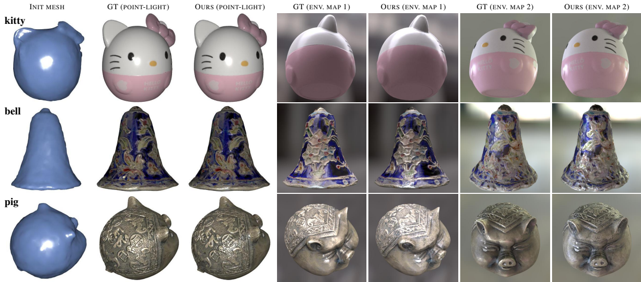
Figure 9: Reconstruction results using synthetic inputs: We obtain the initial meshes (in the left column) using Kinect Fusion [NIH* 11] with low-resolution ( 48 \times 48 ) and noisy depths. Our analysis-by-synthesis pipeline successfully recovers both geometric and reflectance details, producing high-fidelity results under novel viewing and illumination conditions.
