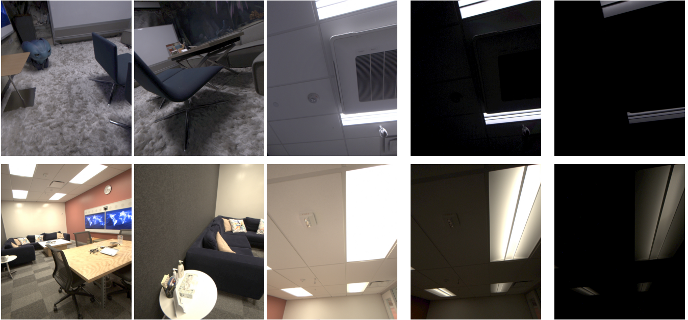
Figure 3: Scenes from the Replica dataset [SWM*19] were captured with a handheld camera rig. The RGB video stream uses multiplexed HDR: SDR frames alternate between three exposure times (1/100s, 1/1666s and 1/16666s). For each camera pose, we therefore have access to a single SDR frame only.
