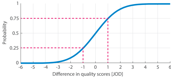
Fig. 2. This plot shows how pairwise comparison preferences are represented in just objectionable difference (JOD) scores. For example, if a distorted mesh A is 1 JOD away from the reference, this represents a 50% decrease in likelihood of selection, i.e. the reference will be chosen over A 75% of the time. More detail can be seen in Sec. 3.9 of the work of Mantiuk et al. [2021].
